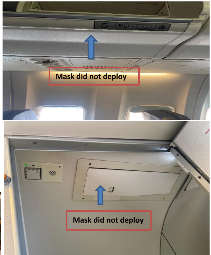
Fig 4: Seat no. 5 mask did not deploy (above); LAV A mask did not deploy (below)
