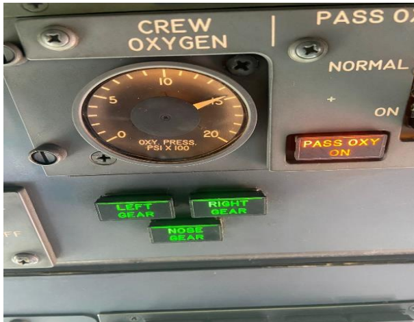
Fig 5: Crew oxygen pressure level after occurrence
